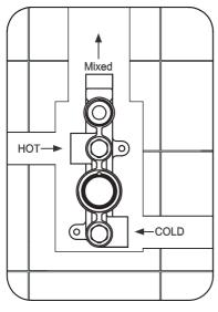
Prepare pipes in wall to connect to shower, with cold on the right.
